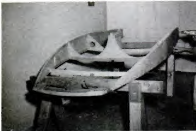
BOAT CAN BE BUILT on two sawhorses with top members parallel; use cord to hold the side planking
